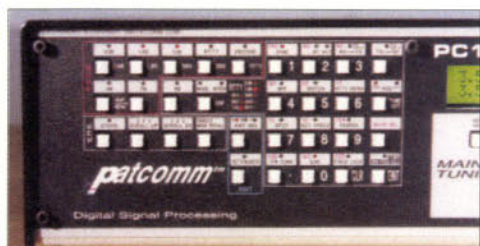
Fig. 1: "The push buttons seem unfinished, with quite sharp edges to them and are relatively close together with very small labelling".
