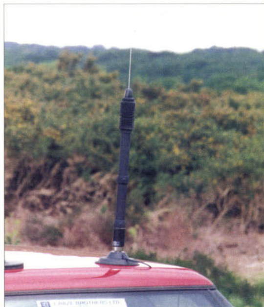
Fig. 6: Close up view of the ATAS-100 automatic tuning antenna system. In use, the motor-driven tuning assembly (within the cylindrical body) is controlled from the FT-100.
