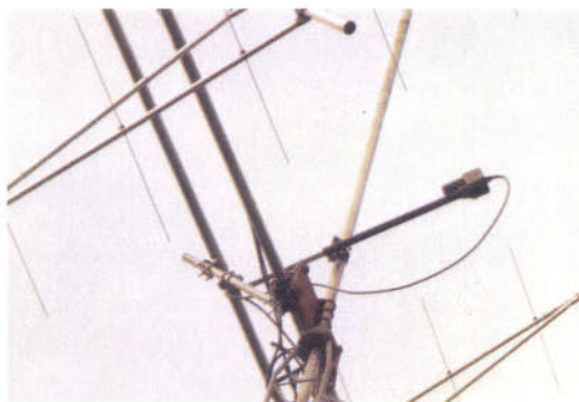
Fig. 5: A satellite 'screw-jack' positioner elevation system up aloft, using a combination of the techniques describe in this article.
