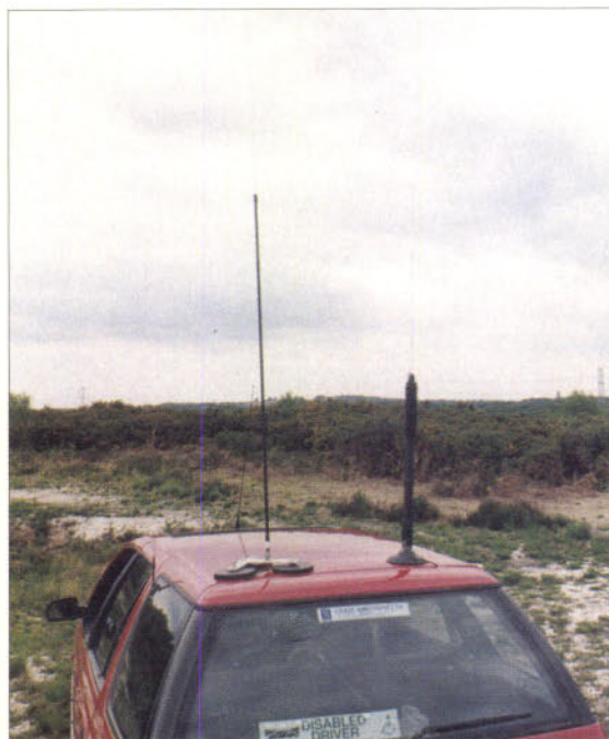
Fig. 5: The Yaesu ATAS-100 antenna unit (right) mounted on G3XFD's car. The antenna on the left is the Pro-AM 14MHz whip. See text for comments regarding 'grounding' techniques.
