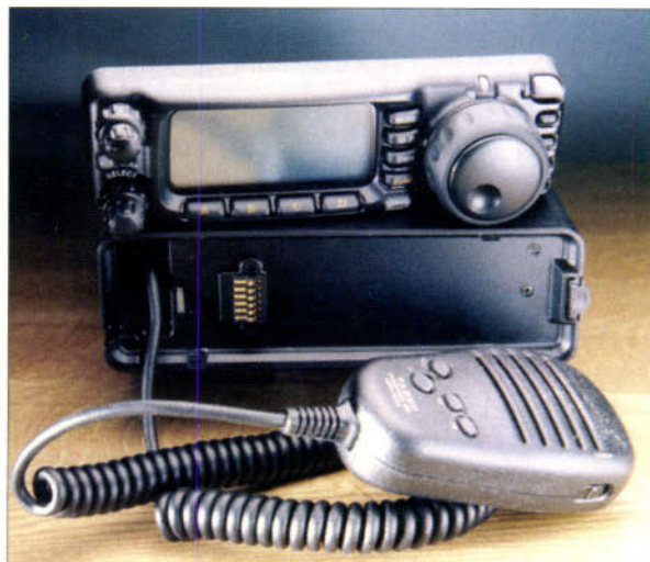
Fig. 1: The front panel of Yaesu FT-100 is completely detachable and uses gold-plated 'wiping' contacts. See text.
