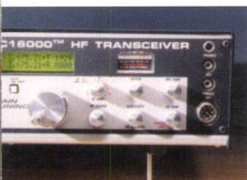
Fig. 2: "The main tuning control is small - it matches the other controls on the front panel, but does not exude quality. The same can be said of the meter, an edge type meter from several years back!"
